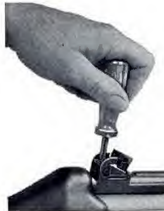
Fig. 38 Loosening the clamping screw
